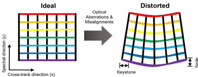
Schematic showing an ideal image compared to a real image with optical distortions [2]
