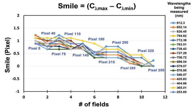
An example of the production testing for HORIBA's hyperspectral/multichannel spectroscopy systems based on the method described above.
