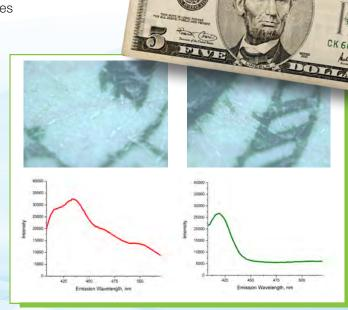
Data from a real and forged US 5 dollar bill. Fluorescence imaging shows no obvious differences. However it is easy to spectrally distinguish the real from a fake bill
