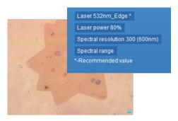
Automatic acquisition parameter selection (spectral range, laser intensity, contrast...)
