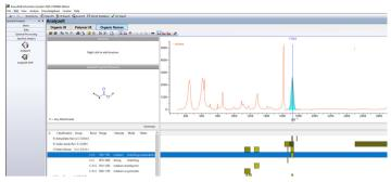
The KnowltAll® environment is integrated within LabSpec 6 Software and contains Single Compound Search, ID Expert multi compounds and SearchIT - once a spectrum has been acquired it will be automatically identified directly in LabSpec.
