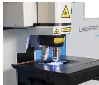
Microlight accessory mounted on LabRAM HR transmission illuminator
