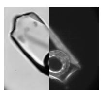
Automatic switch BF / DF diascopic illumination of a geologic solid inclusion with Microlight accessory (50X)
