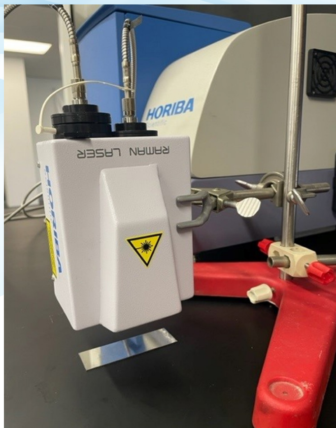
Figure 1: Setup used for acquiring Raman spectra.
