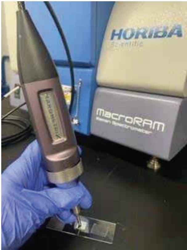
Figure 2: Sample measurement configuration; touch probe connected to the MacroRAM for easy and fast data collection.
