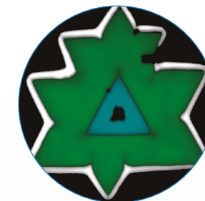
Photoluminescence image of a \text{WSe}_2\text{-WSSe-WS}_2 heterojunction structure
