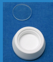
Replacement Spectralon sample cup and coverslip
