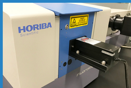
980 nm DPSS laser mounted to the front of the Fluorolog-QM PLQY sample tray
