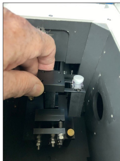
Figure 2: ABS-ACC absorption accessory installed on a standard room-temperature cell holder.
