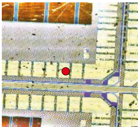
A - Microspot Spot: 1 \mu\text{m} \times 1 \mu\text{m} - Power: 10 mW Power Density: 10 mW/ \mu\text{m}^2
