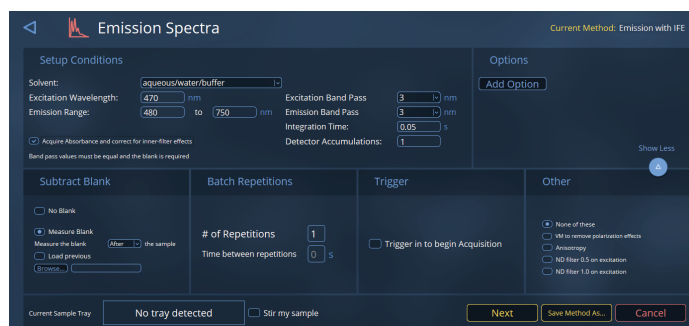
Figure 2: Method for simultaneous acquisition of fluorescence emission, absorbance, and %transmittance spectra with use of inner-filter effect correction in EzSpec software
