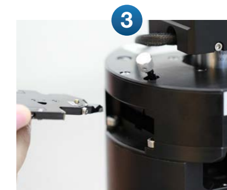
Ease of use: tip replacement Tip replacement without removing the sample or disturbing the optics
