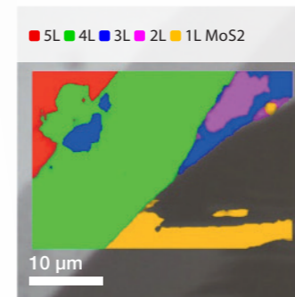
Raman image - Layered MoS 2 structure - Map image was created from low frequency (<30cm -1 ) interlayer peaks
