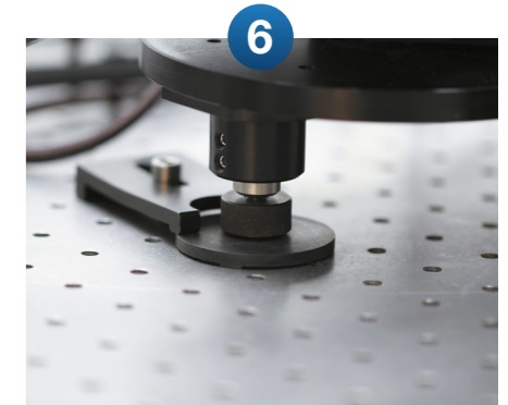
Stability: High resonance frequency AFM scanners High performance without active vibration isolation
