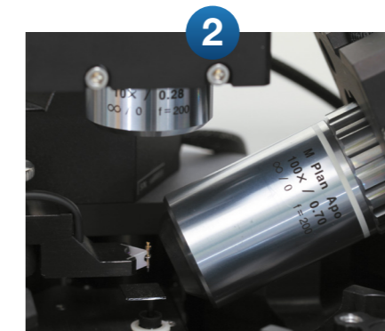
High collection: Wide optical access High numerical aperture objectives for both top and side illuminations
