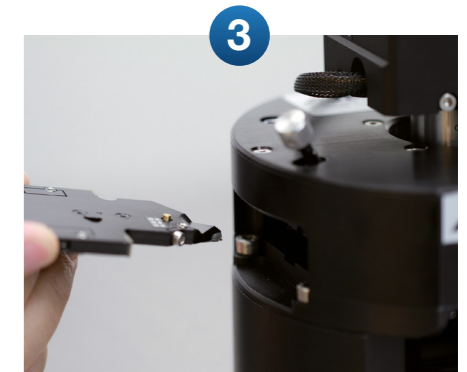
Ease of use: Tip replacement Tip replacement without removing the sample or disturbing the optics
