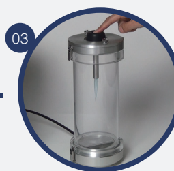
Replace and press the cup to disperse the sample.
