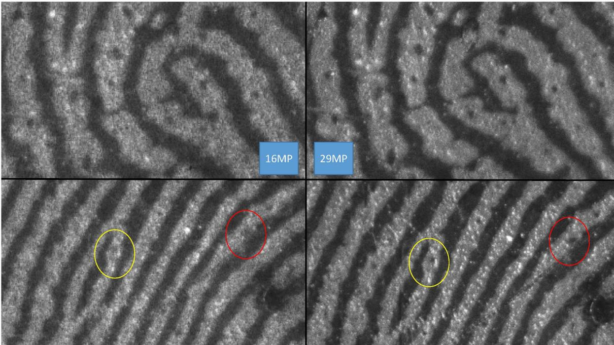
The image above clearly illustrates the difference between an image captured with a 16MP (megapixel) image and a 29MP. With almost double the number of pixels, the 29MP gives a finer resolution. When zooming into a fingerprint ridge, the 29MP shows pores which are missed with a 16MP camera image. The small pores are clearly visible.
