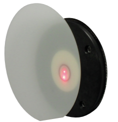
With a transparent Sapphire sample the two DiP beams can be observed.
