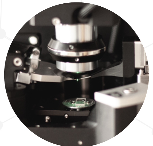
Probe and near-field antenna, with sample retracted
