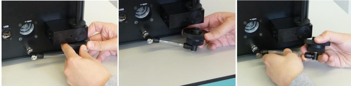
Figure 29: (A-C) Removing the filter holder
