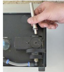
Figure 34: Removing the aerosol guide tube
