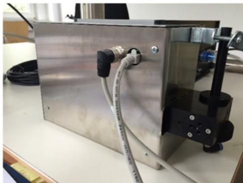
**Figure 2: External aerosol sensor unit APDA-372 E**
