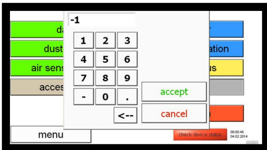
Figure 15: Password entry for accessing the Expert User menu
