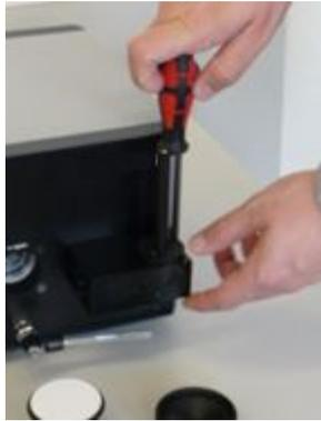
Figure 33: Unscrewing the M3 Phillips head screws
