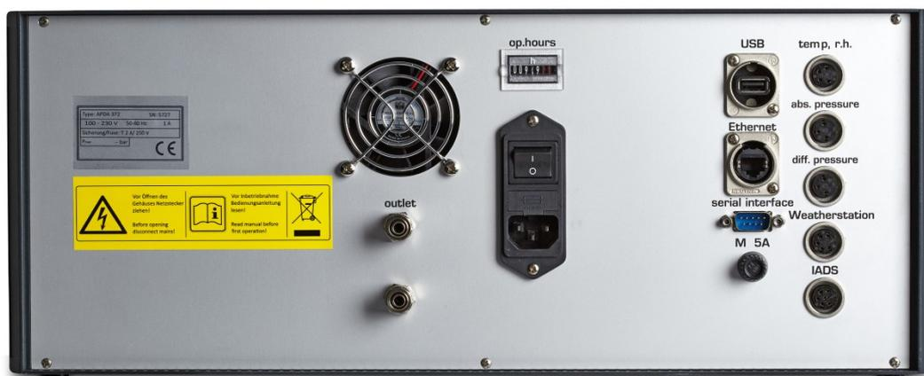
Figure 4: Back of the APDA-372 control unit
