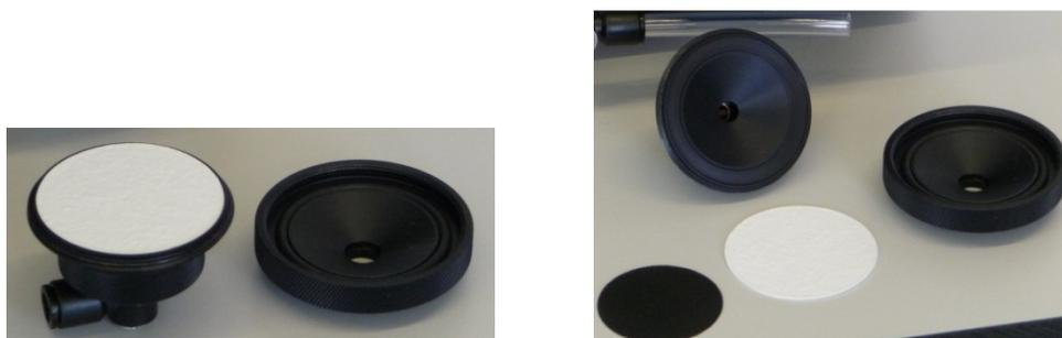
Figure 30: (A and B) filter holder assembly
