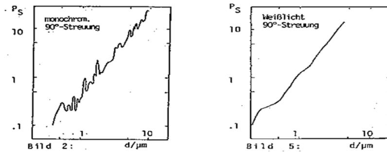
Figure 46: Calibration curve for 90° scattered light detection
