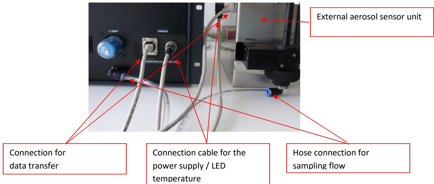
**Figure 6: Connection of the external aerosol sensor unit**
