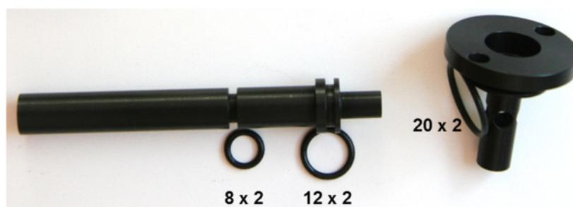
Figure 43: Aerosol inlet, sensor inlet
