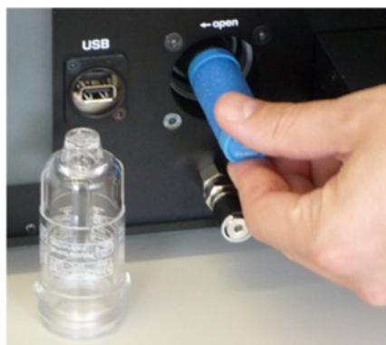
Figure 39: Removing the filter
