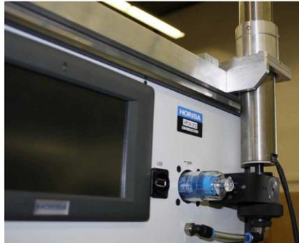
Figure 12: Internal mounting of the sampling tube
