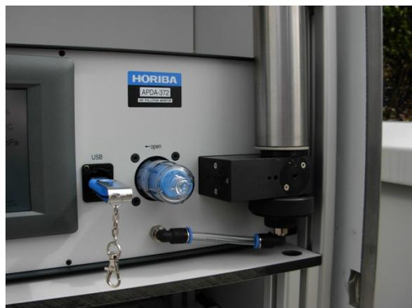
Figure 54: APDA-372 control unit, aerosol sensor with IADS
