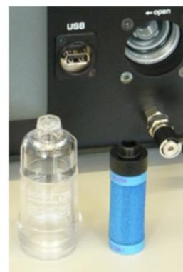
Figure 40: Filter and protective cover after removal
