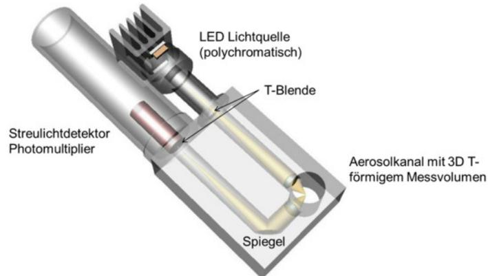
Figure 44: Sensor setup of the APDA-372 measurement system
