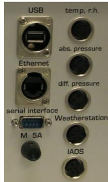
Figure 5: Connections on the back of the APDA-372 control unit
