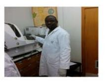
400 Chemistry analyser to learn calibration more on curves. Beer-Lambert Law, accuracy and precision. Students are able to use the instrument's precision check function to statistically cross check results attained using manual *spect*roscopic methods. "In response to requests from employers, we are able to ensure that our students are fully grounded in quality control issues and measures, such as Levey-Jennings Charts and Westgard rules,' Yvonne commented Elliott.
