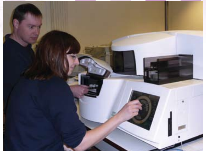
The ABX Pentra 400 benchtop chemistry analyser in the Bulmers Cider Mill analytical laboratory provides user friendly sugar content testing for cider production
