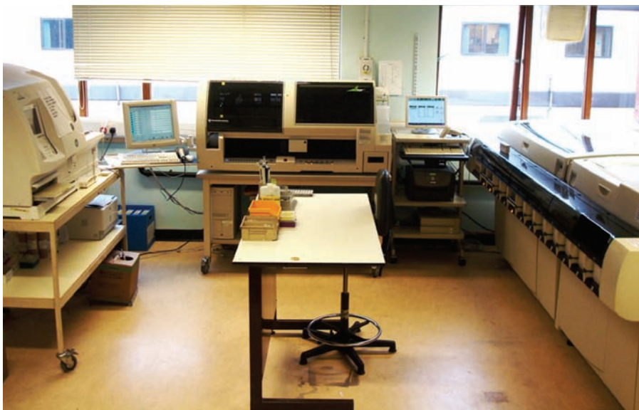
Fig 1. U-shaped Lean analytical work cell at Path Links' Lincoln laboratory.
