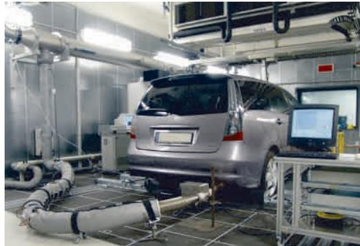
An automotive emission measurement system
