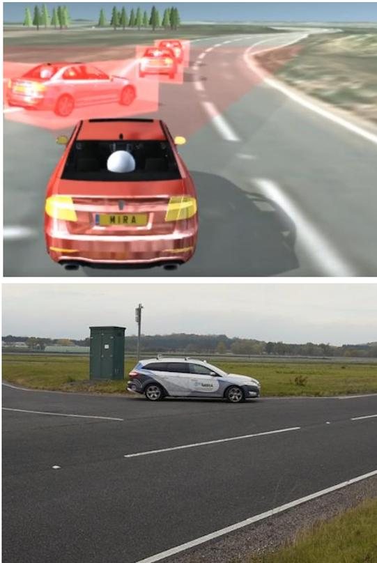
Figure 6 – DigiCAV test of a CAV control systems in a cooperative traffic merge scenario. As seen in DigiCAV's 3D visualisation tool (top) and on the proving ground (bottom).
