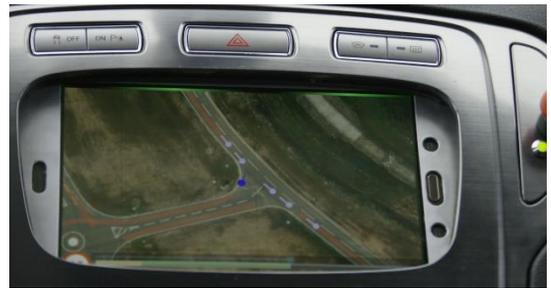
Figure 7 - Cooperative merge test scenario as observed from within the NGV. The current location of the NGV and other test agents is visualised on the NGV's user interface.
