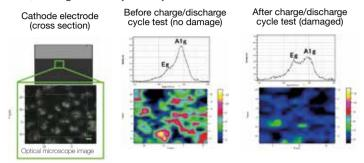
Mapping shows the degradation of the cristallyne structure to an amorphous one with charge/discharge cycle through ratio A1g/Eq ratio. Mapping of the intensity ratio gives the effect over the cathode surface thus related to the optical image.
