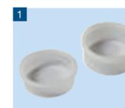
Pour the plating solution into a cell.
