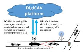
Figure 3 – Vehicle-in-the-Loop scenario with a single vehicle and simulated actors/infrastructure.
