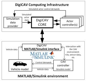
Figure 2 – CAV controller Model-in-the-Loop (MiL) simulation using DigiCAV.
