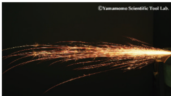
Figure 1 JIS G 0566(1980) Spark test method for steel.*
