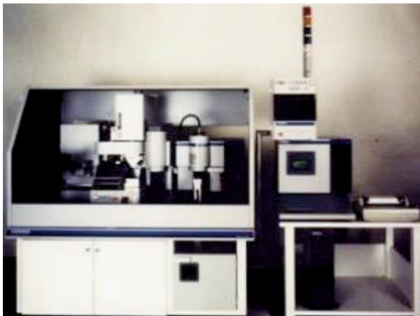
Figure 6 Automated system EMGA-730 with automatic weighing function.
