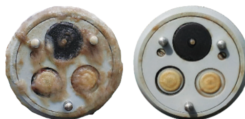
Figure 3 Effect of ultrasonic cleaning on Ammonium Probe: Without (left) and with (right) cleaner after 60 days. https://static.horiba.com/fileadmin/Horiba/Products/Water/Download/Brochures/HAE-T0257.pdf
