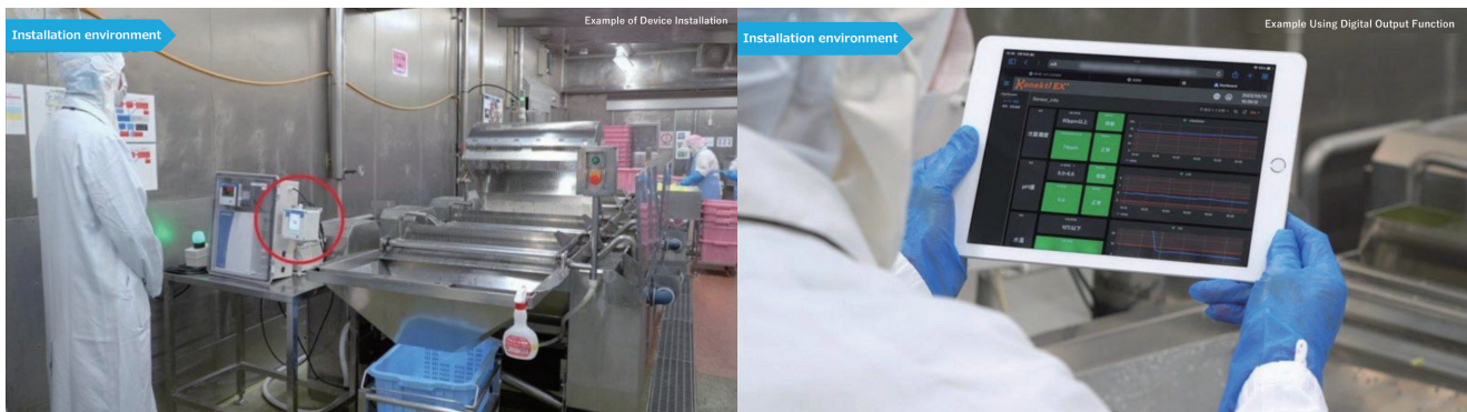
Figure 5 Example of residual chlorine concentration monitor operation at a vegetable processing factory.
