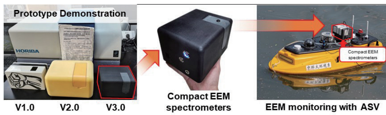
Figure 3 Homemade compact EEM spectrometers
