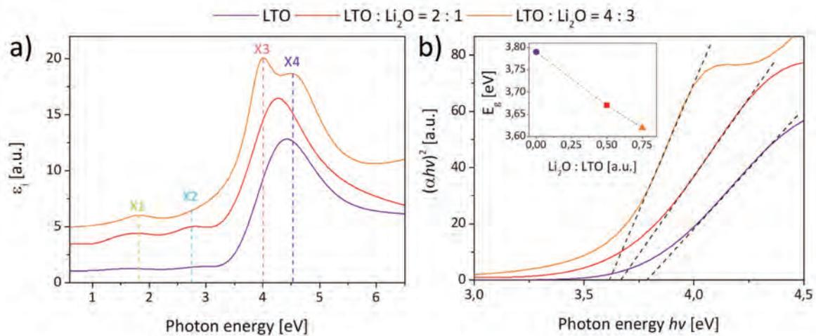
Figure 4 Imaginary part of the permittivity  $\varepsilon_2$  for LTO thin films for different LTO : Li<sub>2</sub>O ablation ratios in (a). Vertical dashed lines indicate significant changes in absorption bands upon lithium addition, marked and color-coded according to X1 – X4. In (b) the evolution of the band gap for different LTO : Li<sub>2</sub>O pulse ratio (as inset) are shown.
