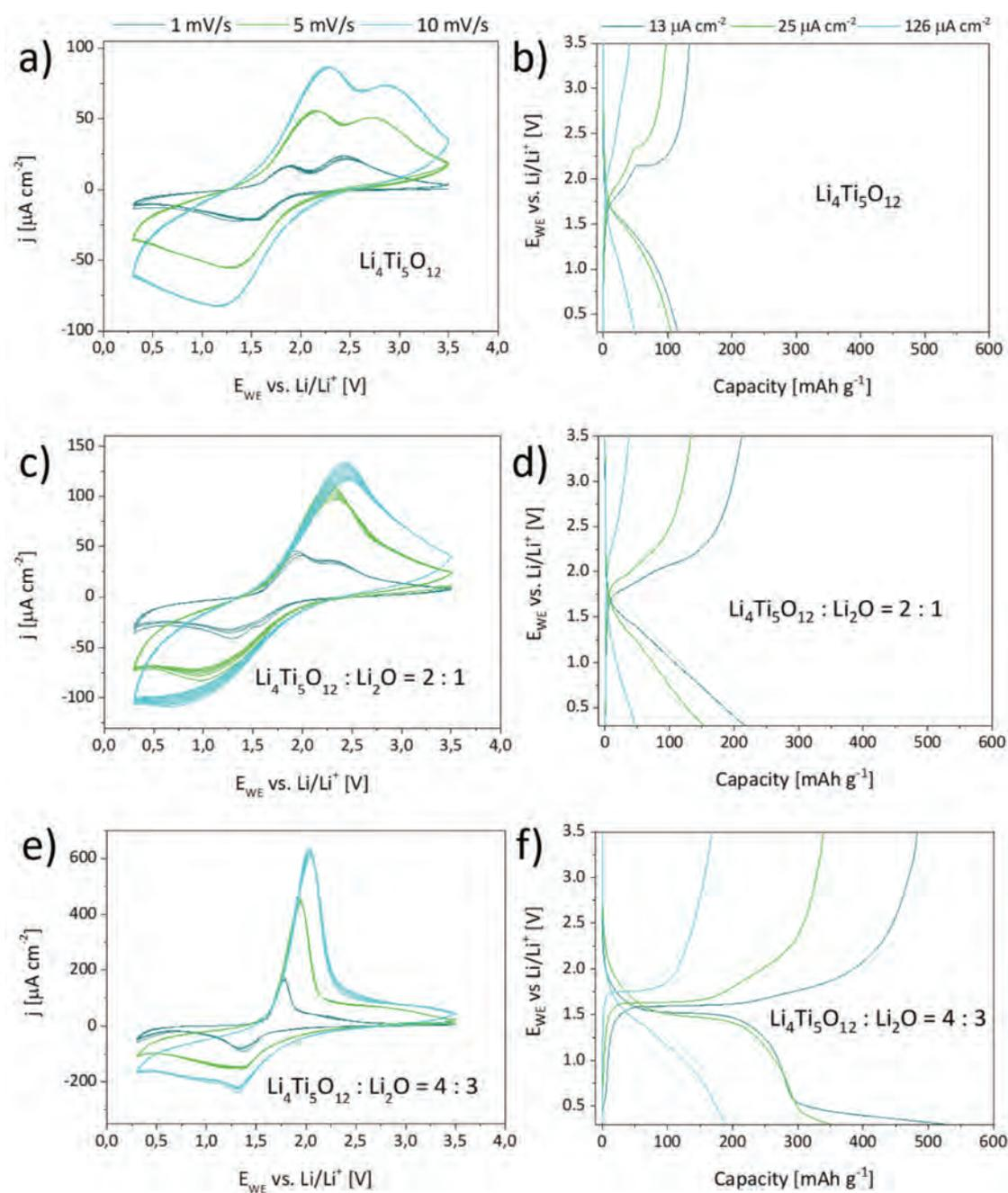
Figure 5 Cyclic voltammograms (left) and constant current charge/discharge curves (right) of LTO layers without additional  $\text{Li}_2\text{O}$  in (a,b) and with additional  $\text{Li}_2\text{O}$  in a pulse ratio of 2:1 (c,d) and 4:3 (e,f) for LTO :  $\text{Li}_2\text{O}$ , respectively. The electrochemical window ranges between 0.3 – 3.5 V vs.  $\text{Li}/\text{Li}^+$ . The applied current densities are  $13 \mu\text{A cm}^{-2}$ ,  $25 \mu\text{A cm}^{-2}$  and  $126 \mu\text{A cm}^{-2}$ .
