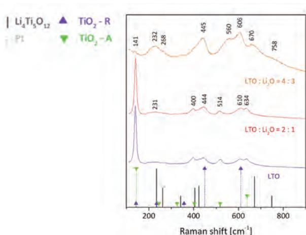
Figure 2 Raman spectra of LTO thin films with different amounts of additional  $\text{Li}_2\text{O}$ . Growth conditions are indicated with the deposition pulse ratio LTO :  $\text{Li}_2\text{O}$ . Raman references for  $\text{TiO}_2$  Rutile and Anatase are from literature.<sup>[1]</sup>
