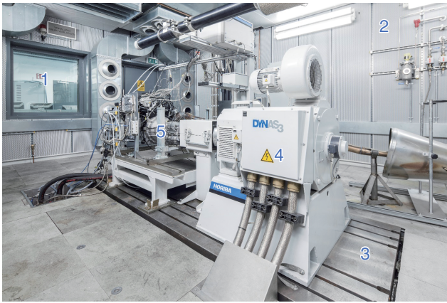
Figure 2 Test cell with TITAN engine test system (HORIBA test center Oberursel, Germany)
