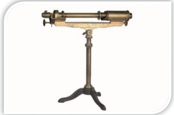
Soleil-Babinet saccharimeter dedicated to the measurement of sugar in blood.
