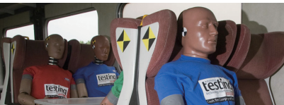
Figure 16 Crash test dummies used in full-scale rail crash testing
