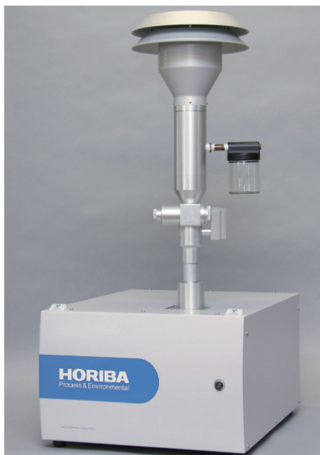
Figure 6 PM2.5 automatic component analyzer
