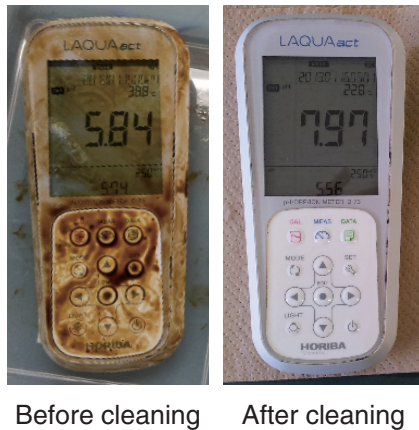
Figure 8 Appearance of LAQUAact (pH meter) with dipping into oil
