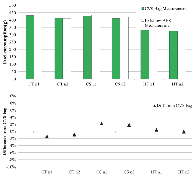
Figure 8 Comparison with CVS carbon balance method (integrated fuel consumption, transient test)
