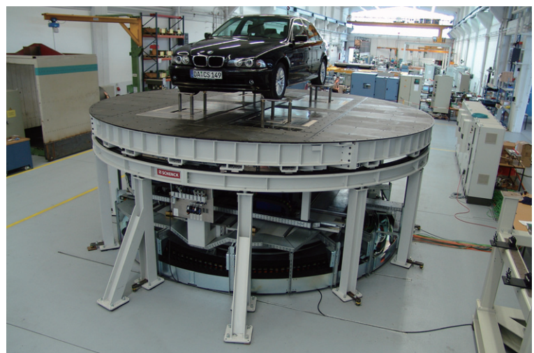
Figure 9 Wind tunnel balance (example)
