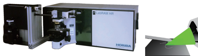
Figure 17 LabRAM HR-AFM coupling system The right picture shows the configuration of incident laser-radiation with 60 degrees angle at samples.
