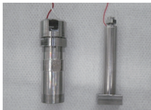
Figure 15 (Left) Previous machined case (Right) New small case
