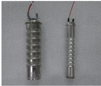
Figure 3 (Left) Standard bellows (Right) Small bellows
