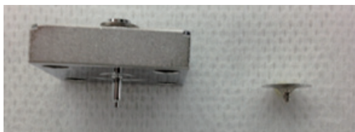
Figure 5 (Left) Standard Diaphragm (Right) Small Diaphragm
