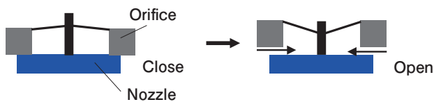
Figure 6 Normally Close valve operating principle
