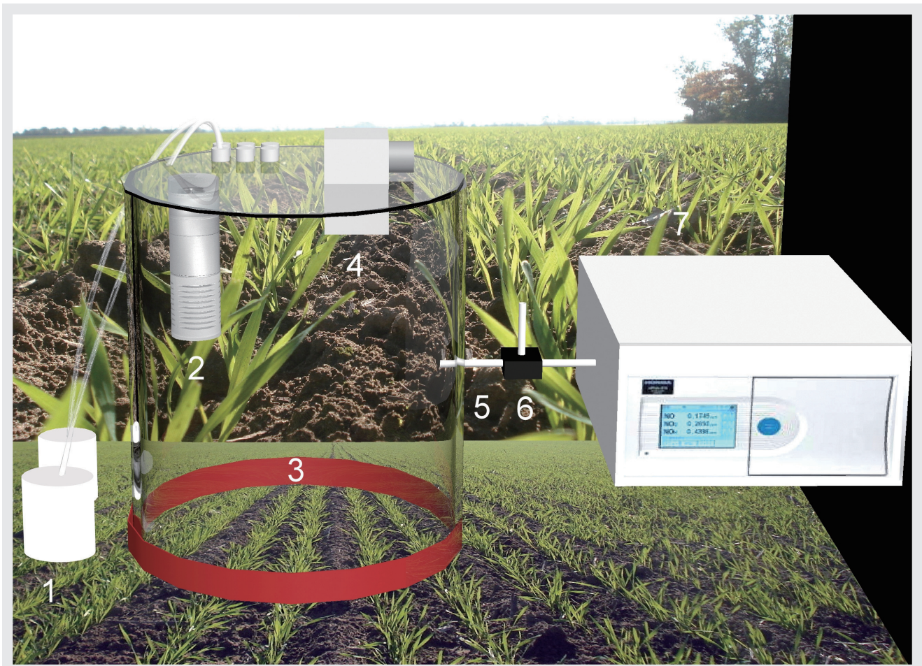
Figure 1 Measuring Setup to Analyse NO-Emissions from Soils. [5]
