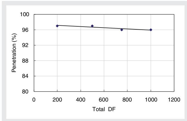
Figure 6 Particle Penetration for All Particles at Different Dilution Factors
