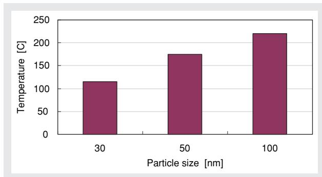
Figure 9 Minimum Temperature for Complete Removal of C40 Particles
