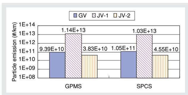
Figure 12 Differences in the Number of Solid Particles Emitted for Each Vehicle
