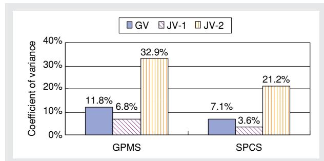
Figure 13 Repeatability of Particle Number Counting Systems (GPMS, SPCS)
