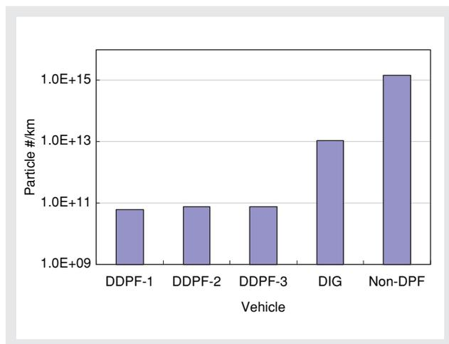
Figure 19 Overall Comparison of Particle Emission in Number / Kilometer from Different Test Vehicles
