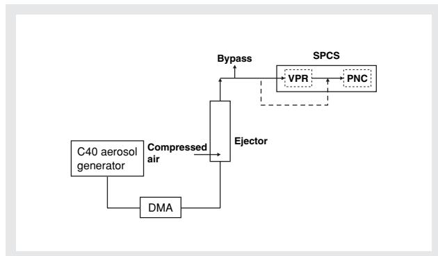
Figure 8 Schematic of Mono-Disperse C40 Aerosol Generator
