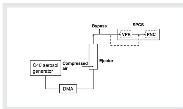
Figure 8 Schematic of Mono-Disperse C40 Aerosol Generator
