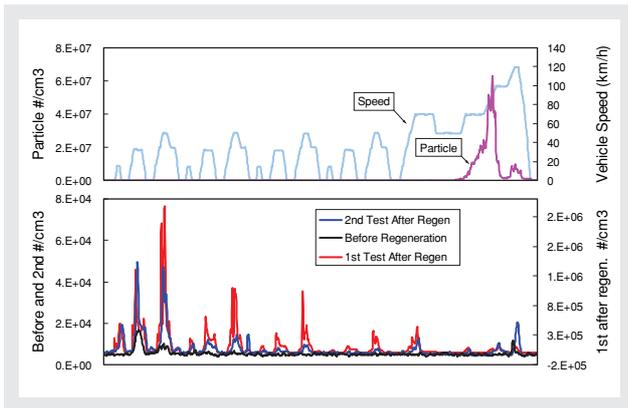
Figure 16 Particle Emission Behavior during Regeneration and after the Regeneration
