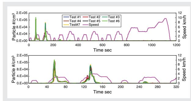
Figure 11 Solid Particle Emission from Golden Vehicle under NEDC Test Cycle
