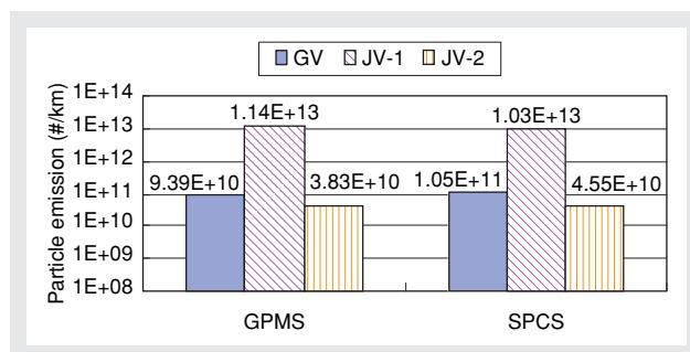
Figure 12 Differences in the Number of Solid Particles Emitted for Each Vehicle
