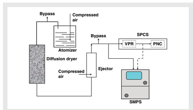
Figure 4 Schematic of Mono-Disperse Particle Generator for Penetration Test
