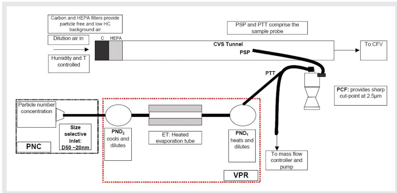
Figure 1 Particle Number Counting System Requirement in UN/ECE
