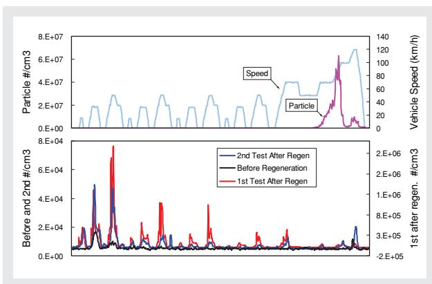
Figure 16 Particle Emission Behavior during Regeneration and after the Regeneration
