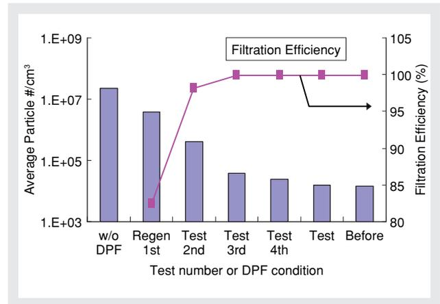
Figure 17 Filtration Efficiency of DPF at Different Situation
