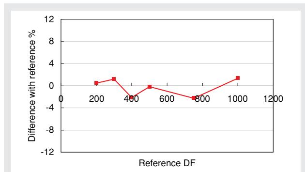
Figure 10 Percentage Difference between the Reference Dilution Factor and Measured Dilution Factors.
