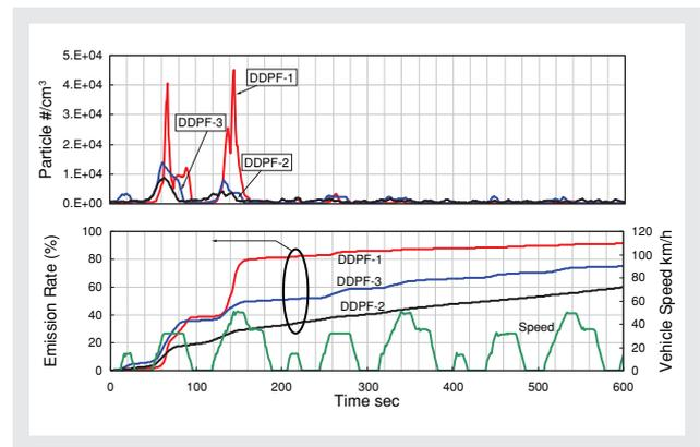
Figure 15 Emission Behavior of Solid Particles from Three Vehicles Fitted with DPF
