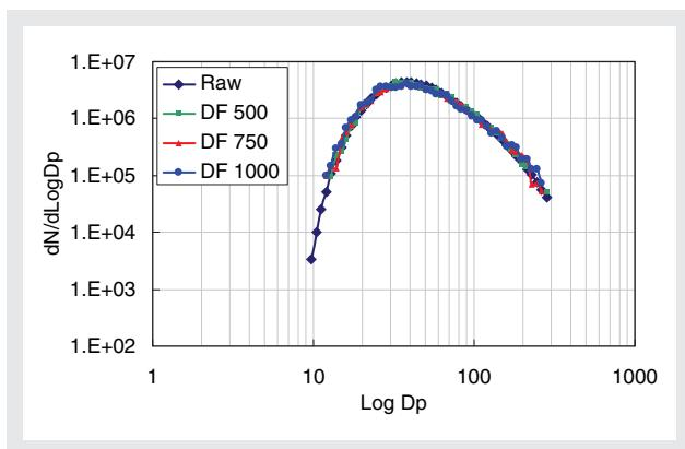
Figure 5 Particle Size Distribution for Different Dilution Factors
