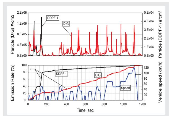
Figure 18 Comparison of the Real-time Particle Emission from DDPF-1 and DIG Vehicles
