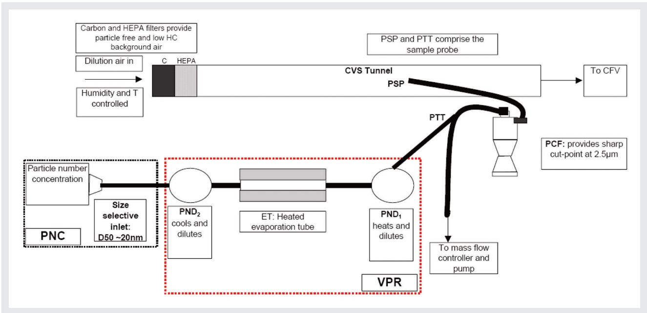
Figure 1 Particle Number Counting System Requirement in UN/ECE
