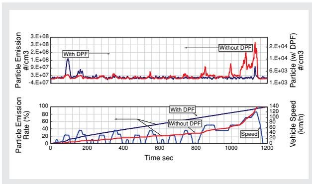
Figure 14 Particle Emission from DI Diesel Engine with and without DPF
