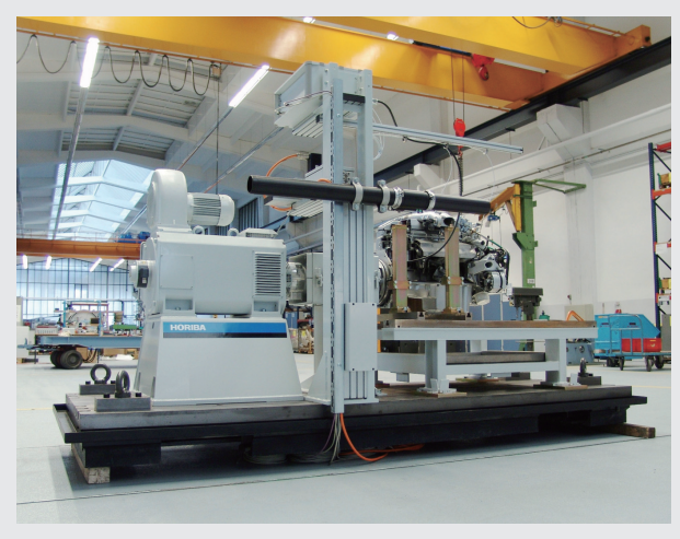
Figure 8 Standard Engine Test System, TITAN
