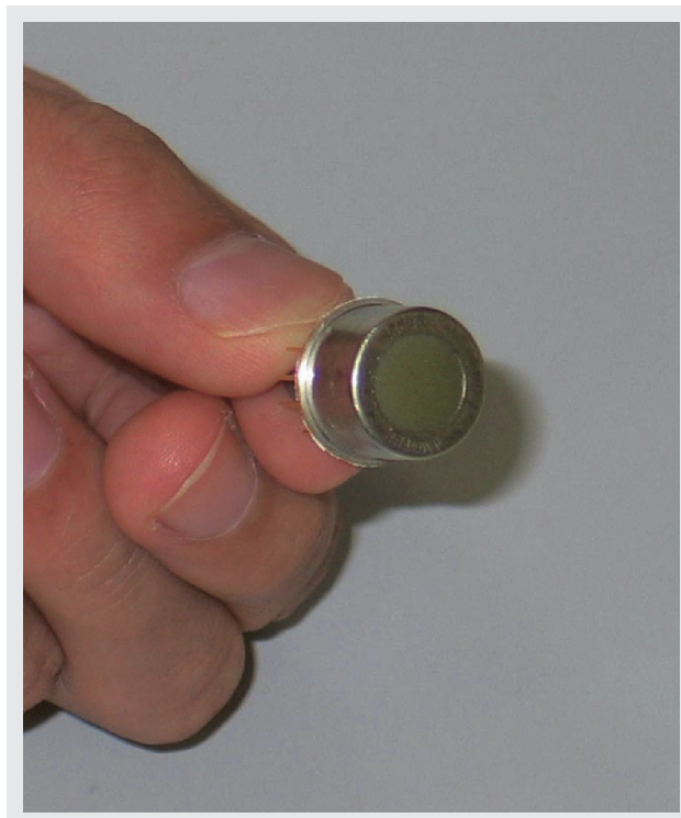
Figure 1 A pyroelectric crystal-type X-ray emitter manufactured by Amptek Inc.
