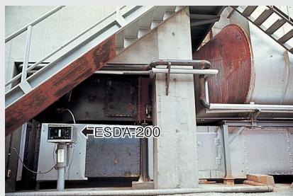
Figure 6 ESDA-200 under Examination Dimensions : 400(W)×550(D)×1200(H) mm Mass : Approx. 60 kg
