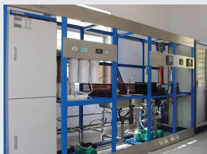
Figure 2 Automatic Measurement Station of Environmental Water Quality at the Shenzhen City's Dam Site in Guangdong Province
