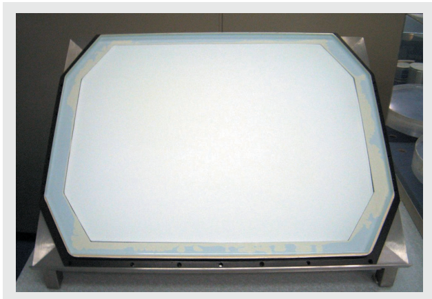
Figure 8 Example of Gamma Plate (480 mm x 550 mm x 9.5 mm)
