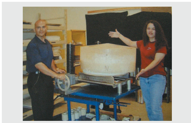
Figure 1 Crystal with a Diameter of 31 Inches (787 mm) and a Weight of 1100 lbs (500 kg)
