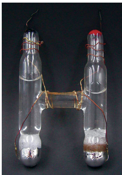
Figure 2 Cadmium Standard Cell (Presented by AIST (National Institute of Advanced Industrial Science and Technology))
