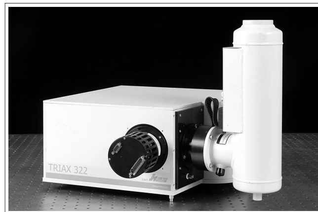
Fig. 2 JY's Unique Dual Array Spectrometer System with a LN 2 Cooled CCD on the Front Port and a TE Cooled InGaAs Array on the Side Port
