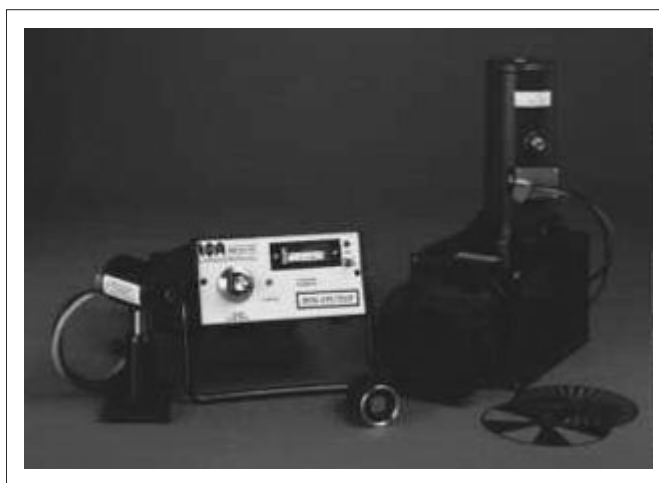
Fig. 4 LN 2 Cooled InGaAs Single Channel Detector
